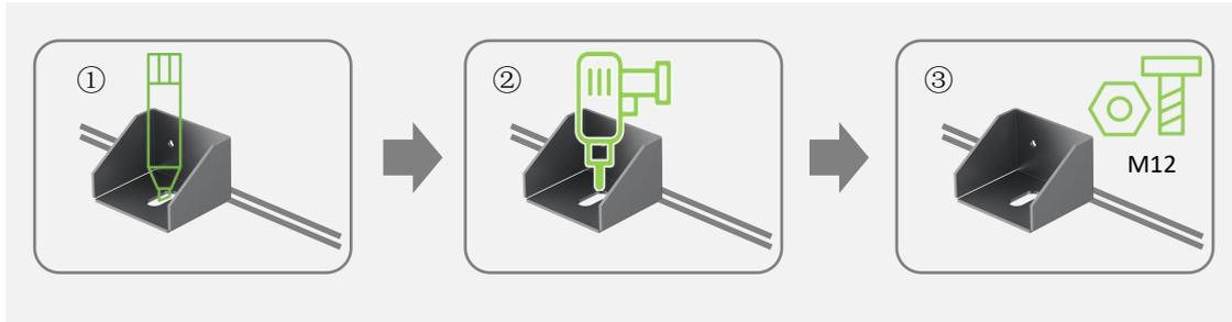
Figure 5-4 Angle Iron Brackets Installation Steps
