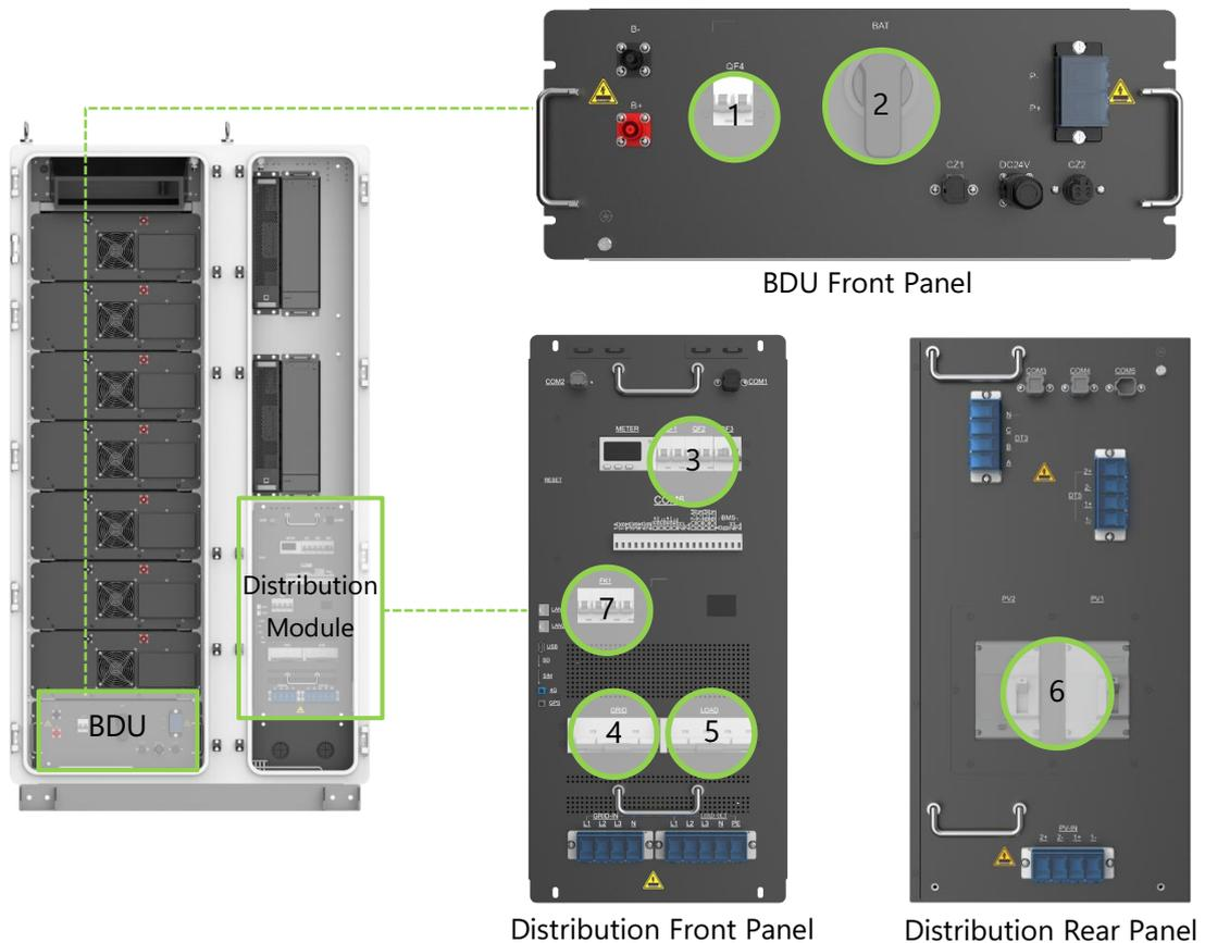
Figure 5-9 Breakers Location
